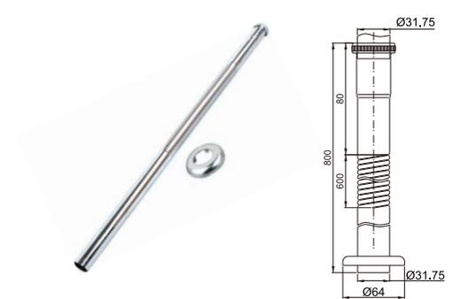
Brass ripple tube Ø31.75
