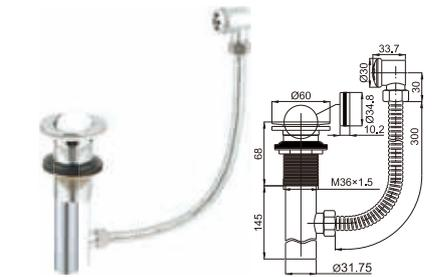
Rotating top waste M36x1.5 with overflow pipe
