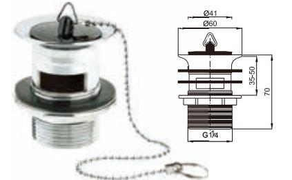
Brass waste for wash basin 1 1/4", with overflow rubber plug with chain
