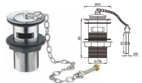
Brass waste for wash basin 1 1/4", with overflow brass plug with chain & screw nut
